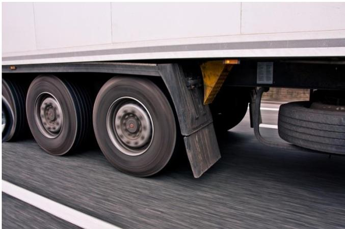
**Tires are responsible for up to 15% of fuel consumption. They use up energy<sup>1</sup>.** This is mainly due to the rolling resistance, which is one of the main forces a vehicle must overcome in order to carry on moving. Vehicle tire manufacturers offer tires of low rolling resistance, which lead to lower fuel consumption and longer tire life. According to tests conducted by Michelin<sup>2</sup>, tires with low rolling resistance can save up to 80 liters of fuel during their lifetime.
